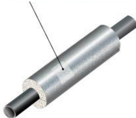
Figure 38 shows the installed 1577CW-EMJ “patch” used to seal the rip in the 3M™ VentureClad™.
