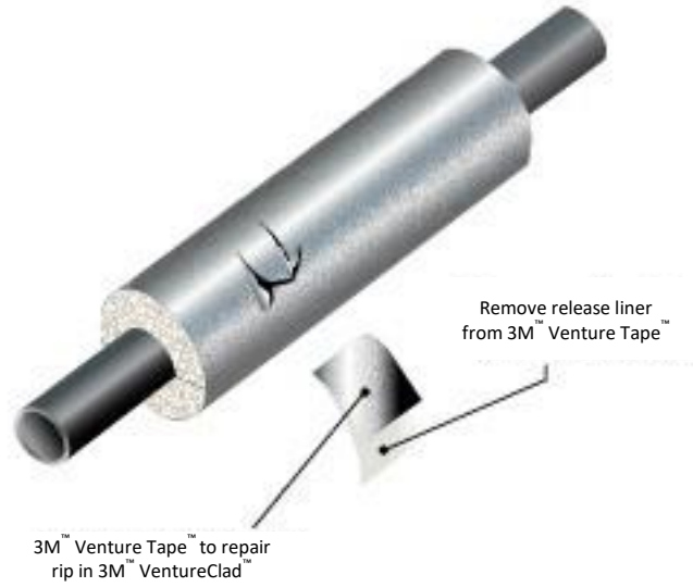
Figure 37 shows taking a piece of 4-inch (100mm) wide 1577CW-EMJ and removing the release liner to allow its application to the 3M™ VentureClad™ surface.
