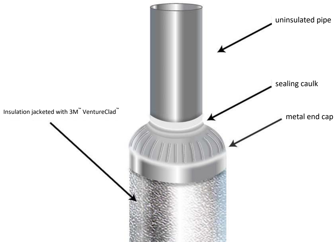
Figure 29 shows a metal end cap installed over a straight section of pipe, jacketed with 3M™ VentureClad™, and a bare pipe above that. The correct installation of the metal end cap, with a sealant, will prevent water from precipitation getting into the insulation.
