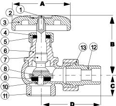
**Specifications:** Designed for residential and commercial use in hydronic applications. Not recommended for use with steam. Seepage feature in seat helps prevent freezing when valve is in the off position. Threaded ends comply with ANSI B1.20.1.
