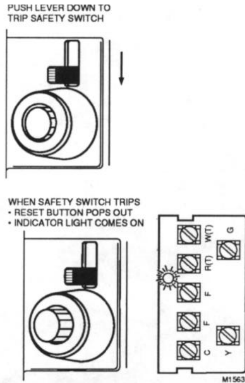
Fig. 6. TRIPPING THE SAFETY SWITCH.
