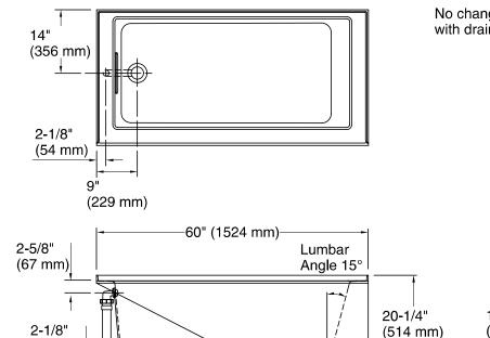
No change in measurements if connected with drain illustrated. (K-7272)
