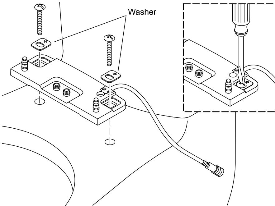
**NOTE:** The following instructions are for toilets without access to the underside of the bowl. Kit 1362736 is required.
