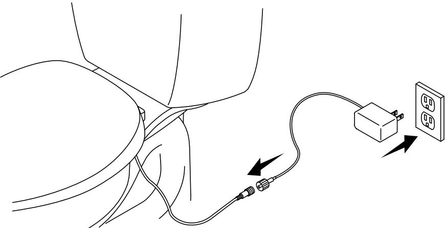
**⚠ WARNING: Risk of electric shock, fire, or personal injury.** Connect only to a nominal 120 VAC, 60 Hz circuit protected by a minimum 15 A Ground-Fault Circuit-Interrupter (GFCI)\*.
