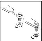
(3) Place side spray holder on mounting hole. Tighten locknut from underneath the sink to secure the side spray holder.
