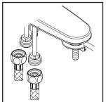
(5) When using stainless steel braided faucet supply hoses; one end of the supply hose is required to have a 1/2" female IPS connection. The other end of this supply hose must match the thread on the water supply valve under your sink. Once you've identified the required size, carefully follow the manufacturer's installation instructions for each hose.
