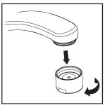
(6) Important: After installation is complete, remove the aerator. Turn on the water and allow both hot and cold water to run for at least one minute each. While water is running, check for leaks. Turn off the water and replace the aerator when finished.
