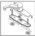
(2) Apply adequate plumbers putty along the boundary of base gasket. Thread mounting bolts to the bottom of faucet. Align faucet with mounting holes and place faucet on the sink, thread locknut onto mounting bolts from underneath the sink, hand tighten locknuts. Go to step (5) if faucet is without side spray.
